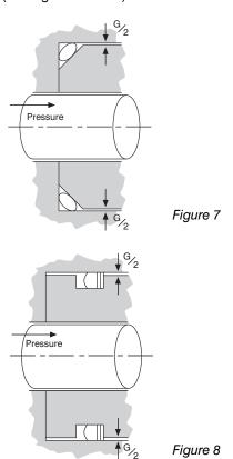
For flange applications, 'O' rings will normally be suitable for sealing pressures above 100bar where metal-to-metal contact prevents extrusion.
