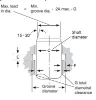
$\begin{aligned} &\text{Max. groove dia.} = \text{C min.} + 2\text{F max.} \\ &\text{Min. groove dia.} = \text{C max.} + 2\text{F min.} \end{aligned}$
