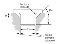
Figure 17: Dovetail groove
