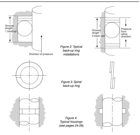
ensure good support. However, they can be scarf split if required, although we do not recommend this because extrusion can occur at the split. Smaller sizes of back-up ring are available only as a single turn. This is because spiral back-up rings need an inside diameter greater than 3mm for machining purposes.
